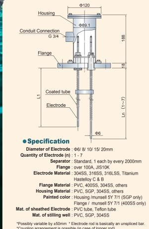
\*Coupling arrangement is possible (in case of longer rod). \*Withstand pressure type can be available. \*Option : Housing, Flange / hot-dip galvanizing.
