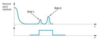
Some applications involve multiple (target + disturbing) echoes even within the measuring window. Basic echo selection will be done by the Quest + software automatically. This parameter influences the echo selection only within the measuring window.
